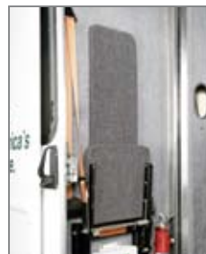
Bulkhead mounted jump seat with optional orange seatbelt
