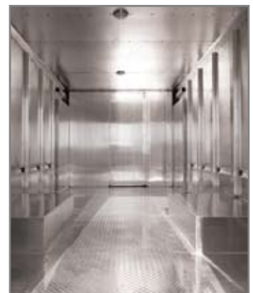
Standard cargo area with smooth aluminum plank floor, aluminum roof liner and optional aluminum diamond-plate overlay and bulkhead separating cab and cargo area
