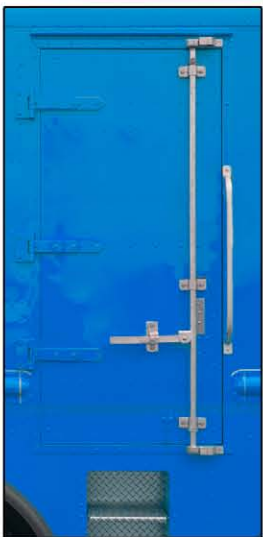
Side cargo doors with Cam Locks
