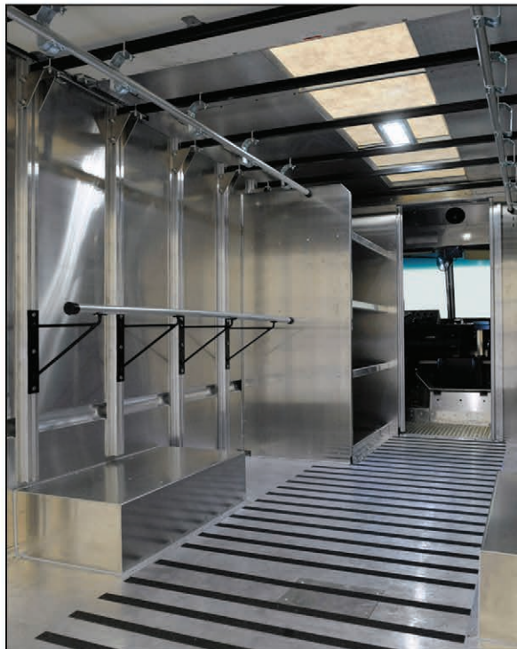
Safety non-slip floor with Twin Uniform Hangers and convenient 4-tier storage shelves ML004, Rev 20B
