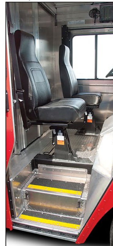
High back vinyl passenger seat w/ wall mounted 3 point seatbelt and SAFETY TREAD steps
