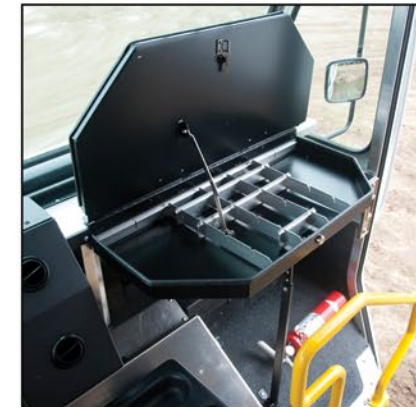
Dash Mounted Work Station w/ dividers and lockable compartment
