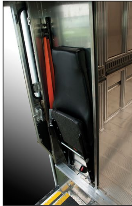
Bulkhead Mounted Jumpseat w/ 3 point safety seatbelt
