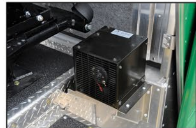
Auxiliary Cab Heater (mounted under drivers seat)
