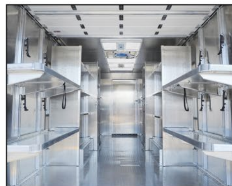
The Center Skylight w/ folding cargo shelves and compartments over the wheel wells
