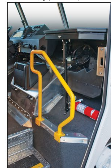
Safety Yellow Grab Rail (fixed) mounted on passenger side toeboard
