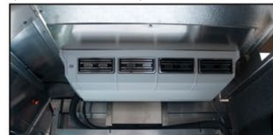
Auxiliary Air Conditioning (mounted over curbside door)
