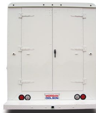
Twin 19 inch Door w/ optional exterior flood lights
