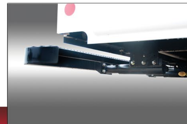
"Best-in-Class" 12 inch Grated Shock Bumper Shock Mounted Bumper w/ "D" shaped rubber
