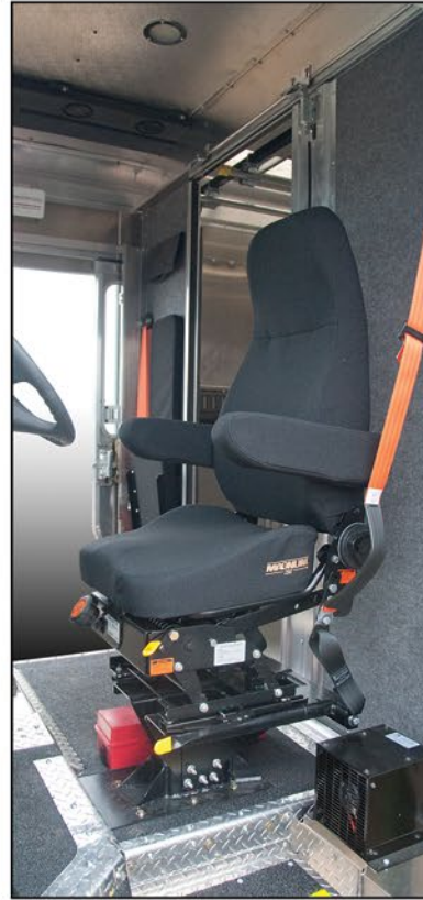
The MAGNUM High Back Mechanical suspension Drivers Seat w/ 3 point safety seatbelt
