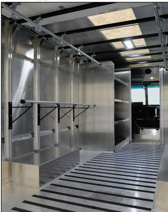
Safety non-slip floor with Twin Uniform Hangers and convenient 4-tier storage shelves ML004, Rev 22A
