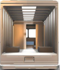
Center Skylight Roof
