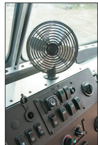
Dash Mounted 2-speed Auxiliary Fan (can be mounted in various cab locations)
