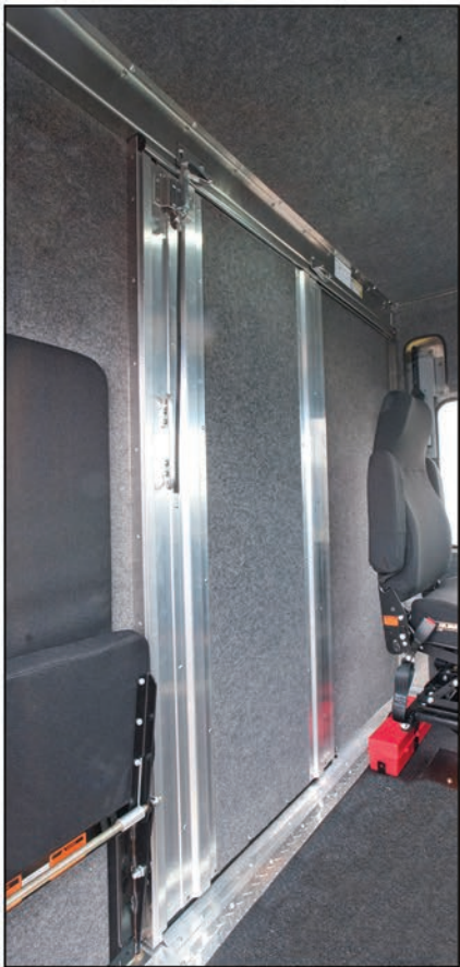
Sound Deadening Material on Bulkhead Panels & Bulkhead Door (cab-side)
