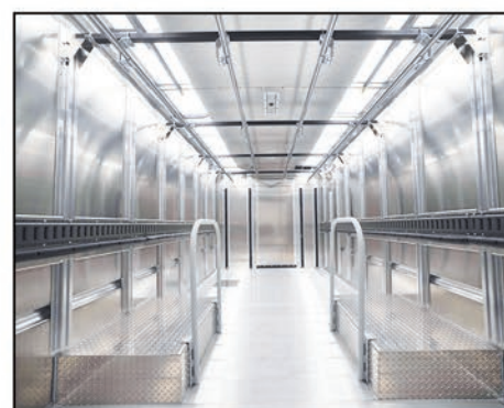
The Split Skylight w/ rug rails over the wheel wells and E-track
