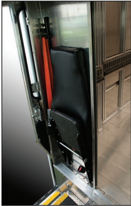
Bulkhead Mounted Jumpseat w/ 3 point safety seatbelt
