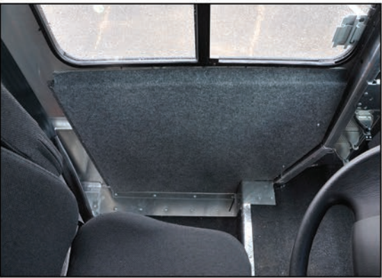
Sound Deadening Material below doorless drivers window
