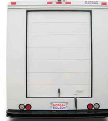
58 inch Roll-up Door w/ Hi Mount S/T/T lights
