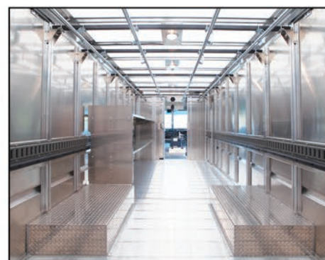
The Full translucent Roof w/ laundry rails and side storage bins also featuring E-track.
