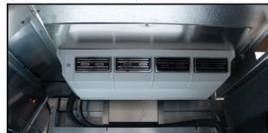
Auxiliary Air Conditioning (mounted over curbside door)
