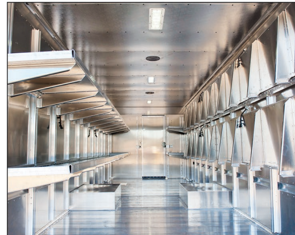
Morgan Olson's Famous Folding Shelf system with our patented infinitely adjustable sidewall stiffeners
