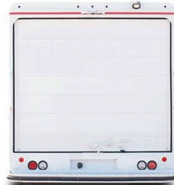
Full Open Roll-up w/ Max Security Latch
