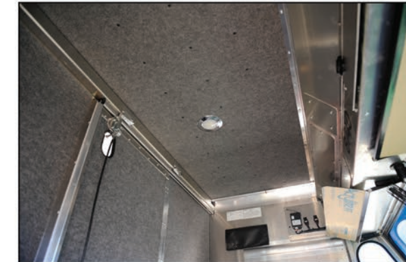
Acoustical Matting provides for a quieter cab
