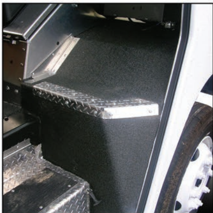
Acoustical Matting on Cab Step Riser and toeboard w/ aluminum diamond plate trim
