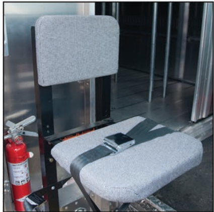
Removable Passenger Jumpseat w/ seatbelt
